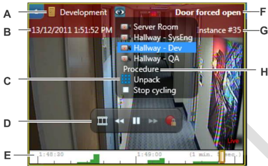
Figure 181. Alarm Management: Active Alarm in Canvas Tile
